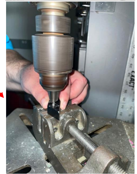
Drill holes on the fiber guider
