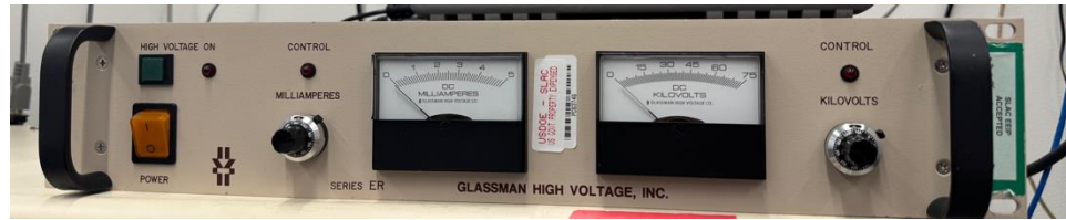
Glassman 75 kV supply
