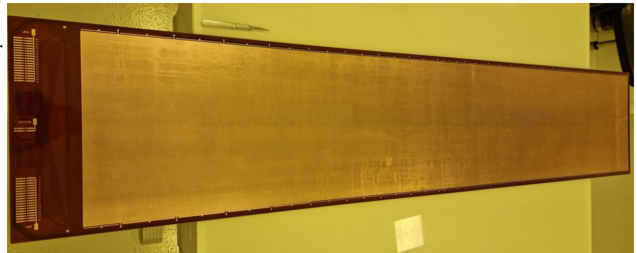
μRWELL / CapaSh readout PCB: Front view
