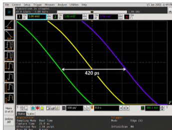
Figure 1: The oscilloscope screenshot shows signals from a synchronous event acquired on three OBDT channels connected to the backend system. The horizontal time scale is set to 100 ps/div.
