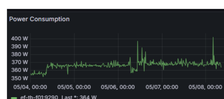
Figure 7: 4U Server Power
