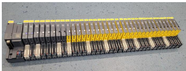
Fig. 8. ET200SP decentralized peripheral module with various I/O modules.
