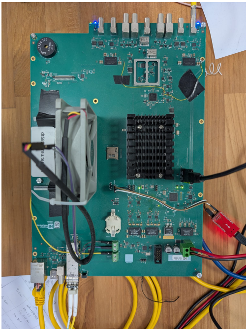
Fig. 7. Prototype board. The central heat sink covers the Zynq UltraScale+ MPSoC; the two LTC2000 digital-to-analog converters and their analog outputs are at the top left, and the 10-gigabit SFP transceiver is at the bottom left.
