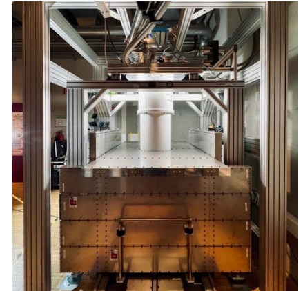
Muon veto: inside and outside the cryostat. Made of 28 plastic scintillator modules with WLS optical fibers and SiPM readout
