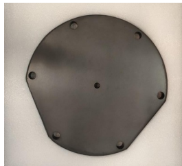
B 4 C: 4 cm of boron carbide for the reduction of thermal neutrons
