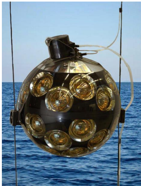
1 Digital Optical Module = 31 PMTs + electronics
