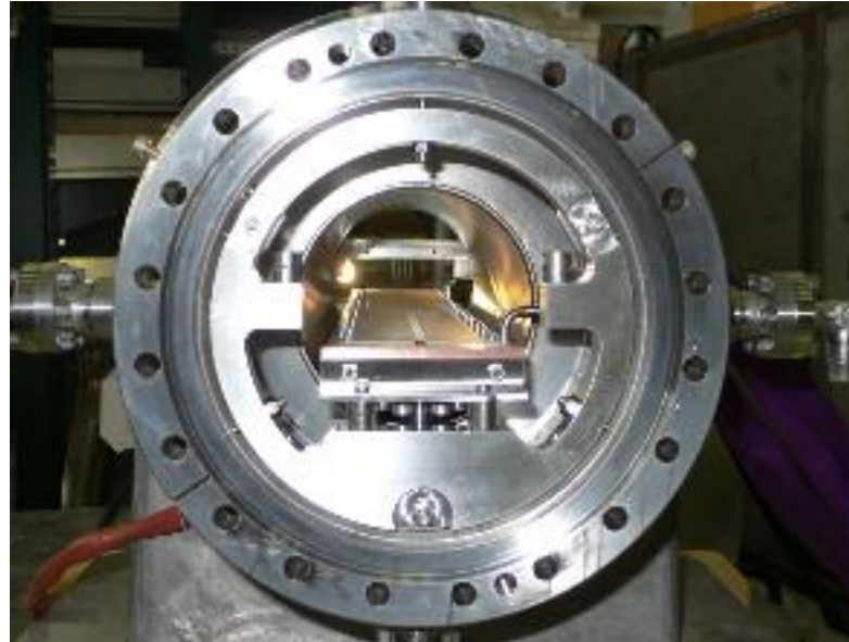
Fast chopper, validated 2013 Risetime < 10 nsec/ extinguish factor 100%
