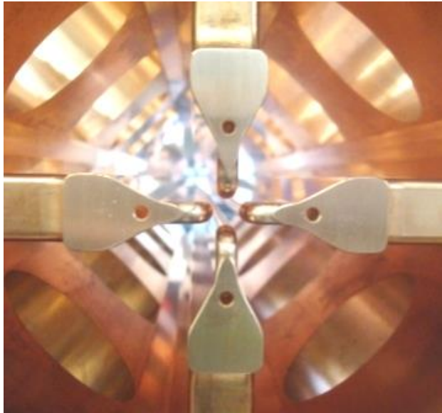
3 MeV/ 352 MHz/ 3 m long RFQ Commissioned with beam 2013
