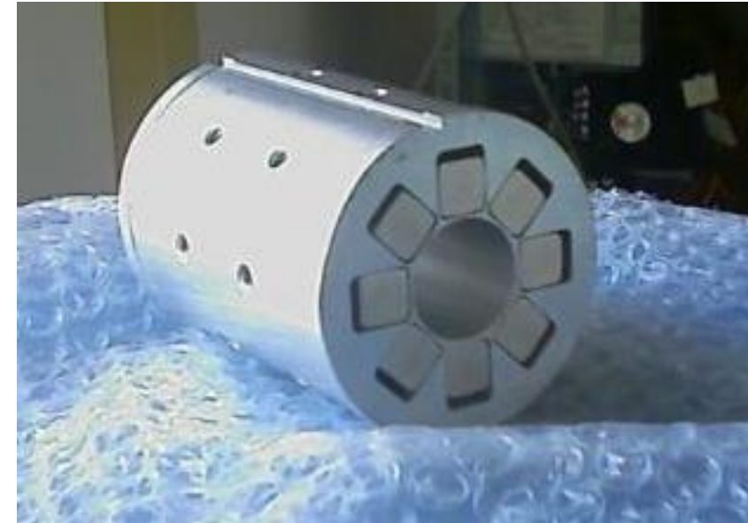
Permanent Magnet Quadrupole for the Drift Tube LINAC, 60 mm in diameter and 80 mm in length Produced in European industry for the first time for LINAC4
