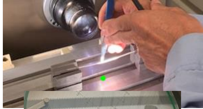
Mandrel inspection and straightening
