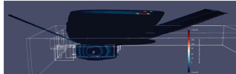
Calculated 3D radiation dose map with no shielding igloo in place
