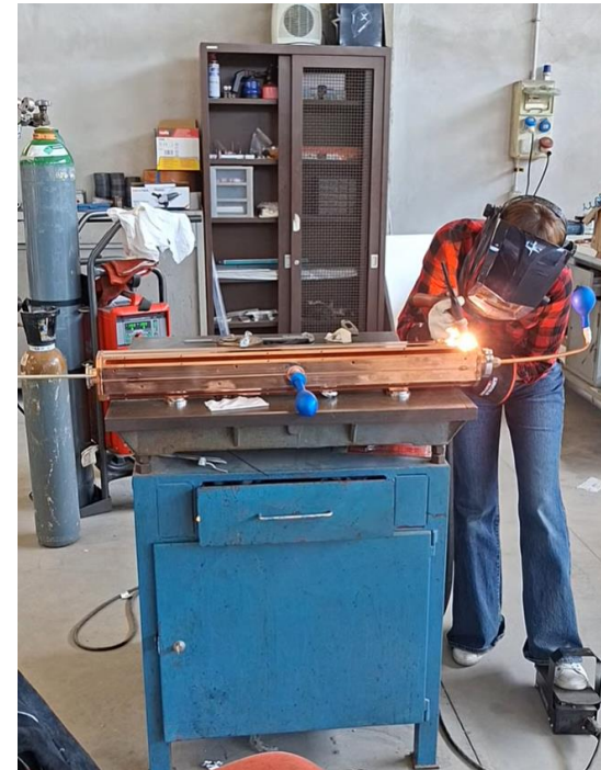
Left: ASTERIX prototype being TIG welded. Right: TIG-welded prototype on the CMM table for mechanical characterization.
