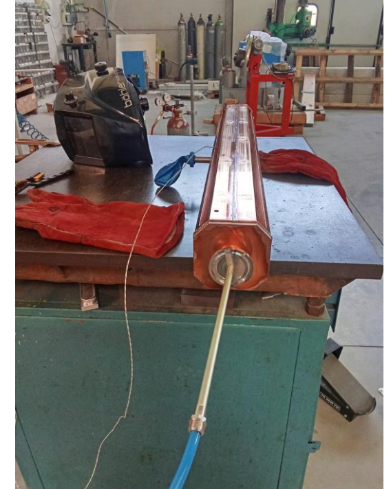
Left: ASTERIX prototype being TIG welded. Right: TIG-welded prototype on the CMM table for mechanical characterization.
