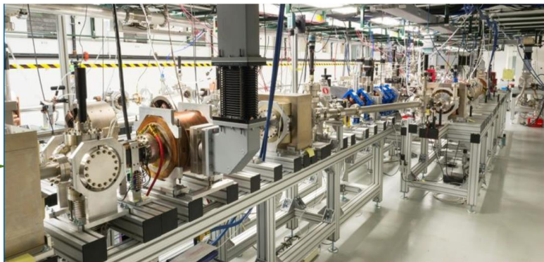
AWA Approach: Requires Stand Alone High-Charge Linac and Power Extraction Transfer Structure (PETS)
