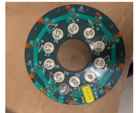
PCB developed to connect multiple 3 He detectors
