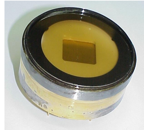
GEM with semi-transparent Photocathode (K-Cs-Sb)
