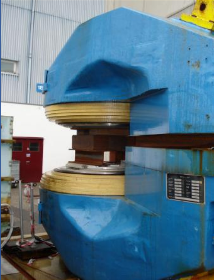
Vertex: MEP48, stored at CERN 400 mm vertical gap Max. field: 1.47 T
