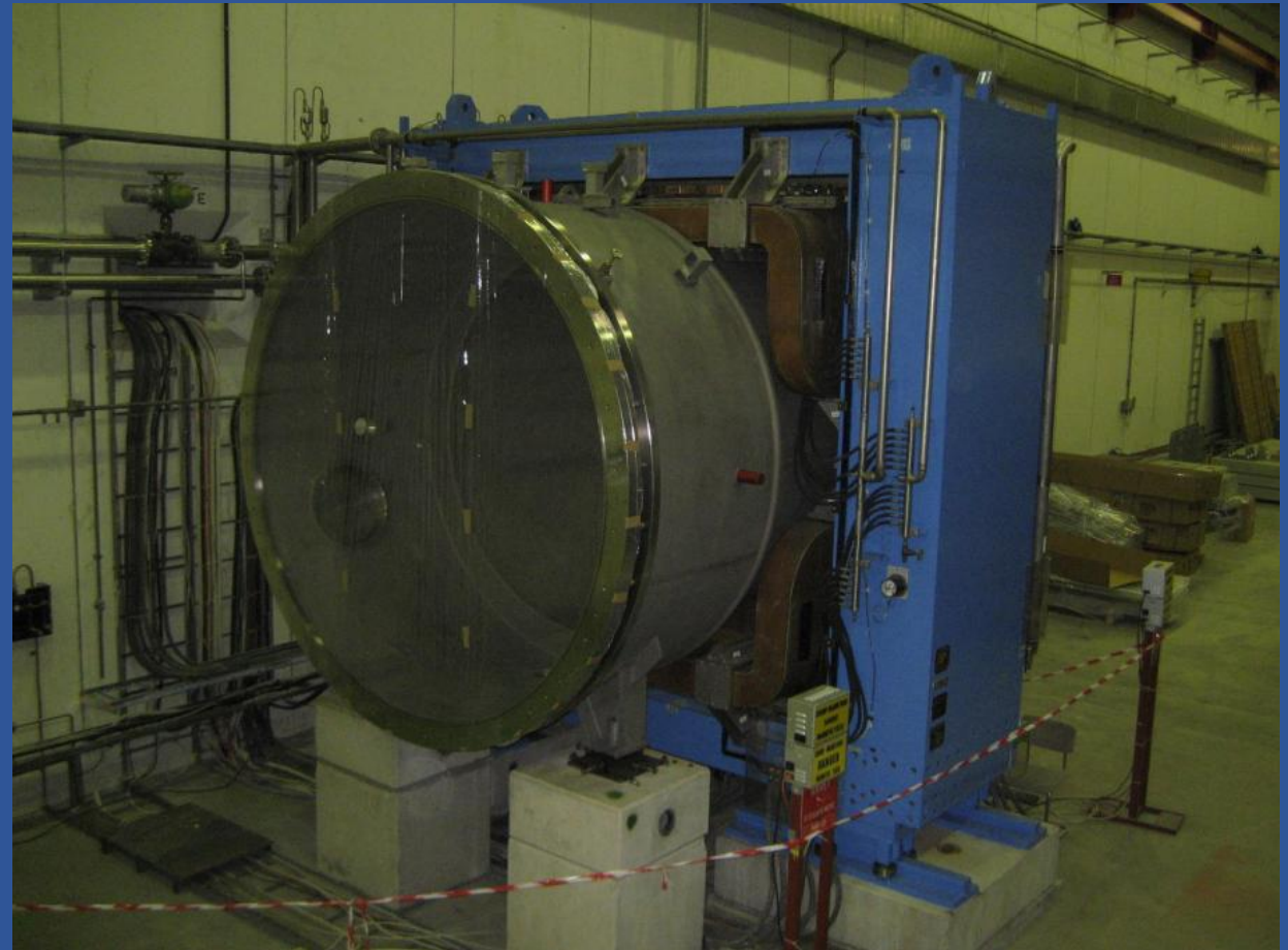
Muon spectrometer: MNP33, in use by NA62 until 2026 2400 mm gap, 2450 mm aperture width 2 coils: 0.9 Tm
