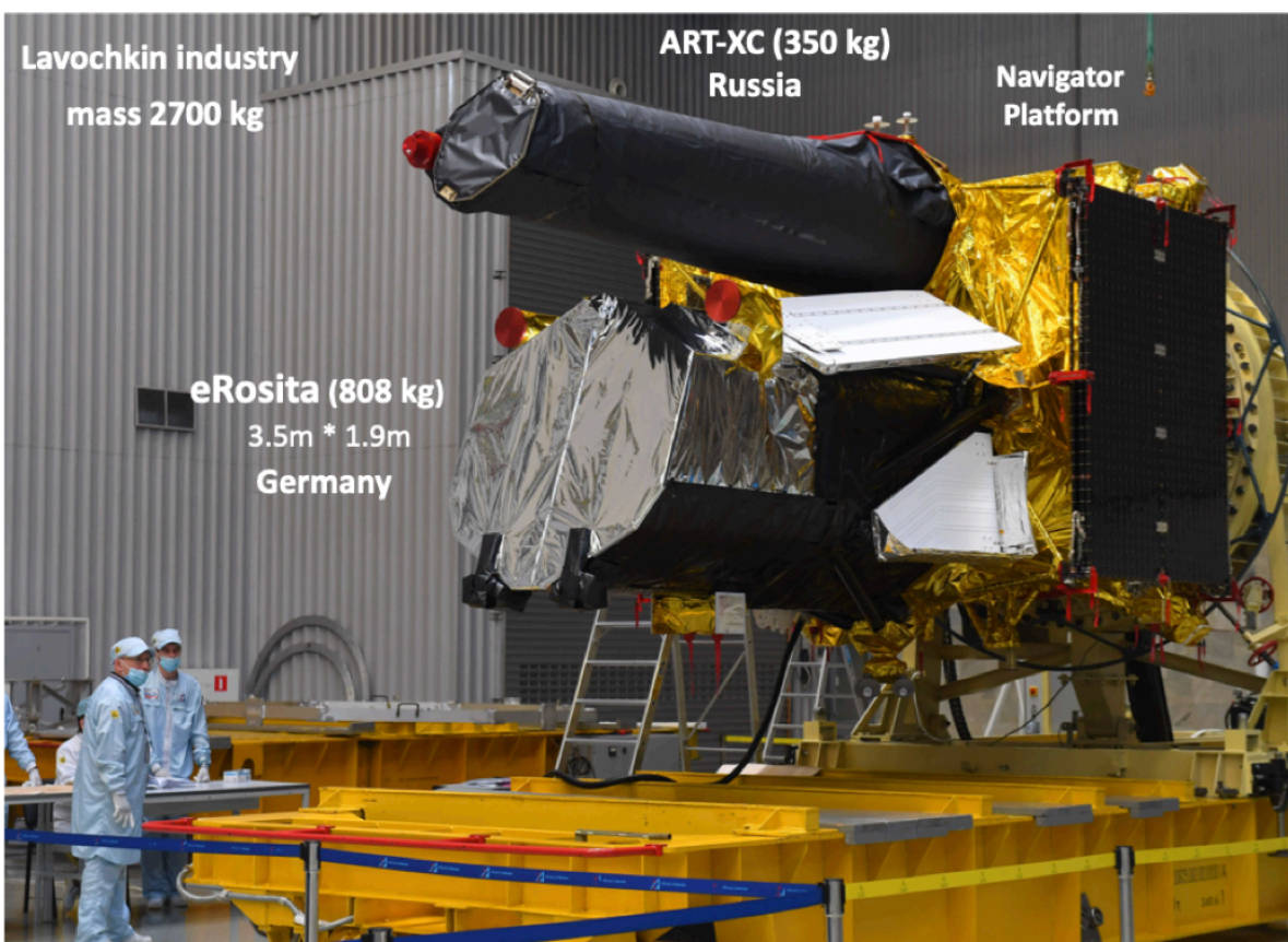
Fig. 2. SRG orbital observatory with the folded solar panels in NPO Lavochkin's assembly hall before shipment to Baikonur.
