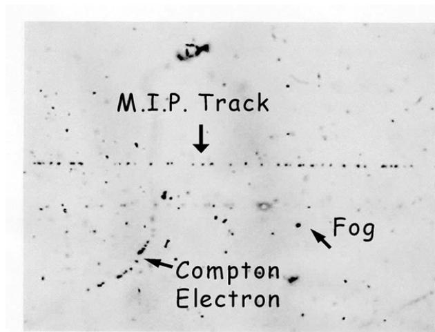
$$-\frac{dE}{dx} = \frac{4\pi z^2 e^4}{m_e c^2 \beta^2} n \cdot \ln \frac{m_e c^2 \beta^2 \gamma^2}{2\pi \hbar \langle \nu_e \rangle}$$
