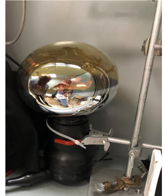
Hamamatsu R5912-100 Water tight assemblies (4 in hand)
