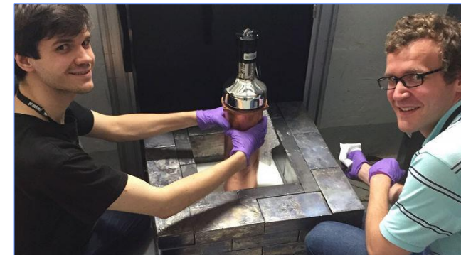
16 kg NaI detector from COHERENT collaboration
