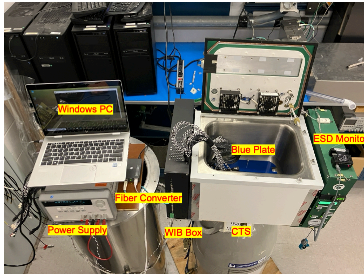
QC Test Setup Hardware
