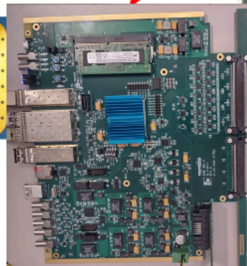
Warm Interface Board (x5) Xilinx Zynq UltraScale+ SOC FPGA (includes ARM cores; can run Linux)
