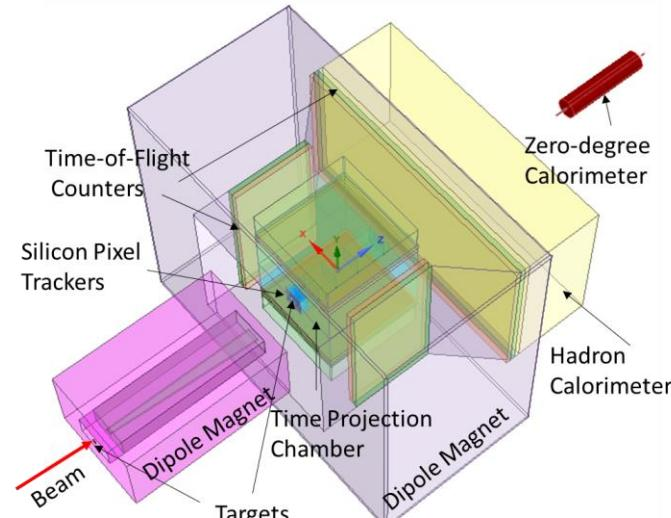
Schematic view of final spectrometer
