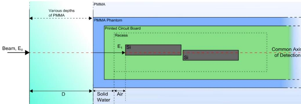
Figure – Schematic of experiment, beam energy  $E_0$  is modified along trajectory through materials & detector to deposit PBP in sensitive volumes for measurement.
