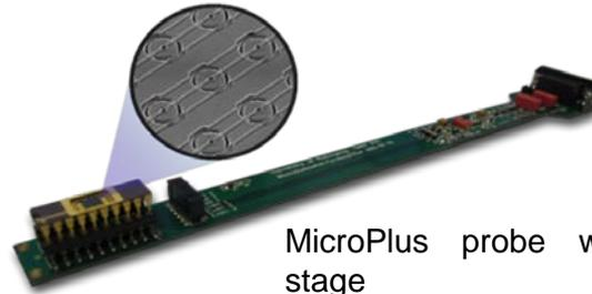
MicroPlus probe with XY-movement stage
