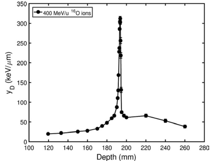
Dose-mean lineal energy measured for 400 MeV/u  $^{16}\text{O}$  ions
