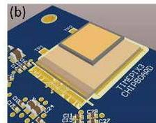
Sketch of Diamondpix. (a) CVD diamond layer is bump bonded on the Timepix3 chip which is fixed on a (b) standard Timepix readout board. Figure reproduced from Claps, et al, 2018.
