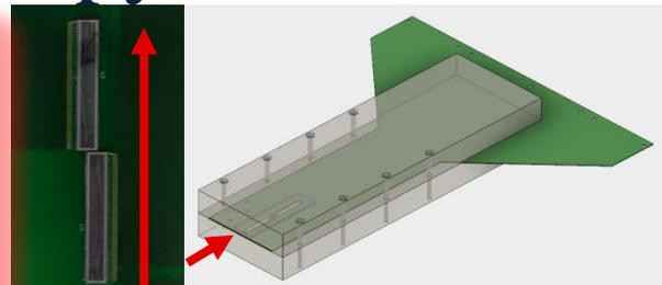
(Left): Photograph of sDMG linear array of detectors. An arrow indicates the direction of the axis of detection.
