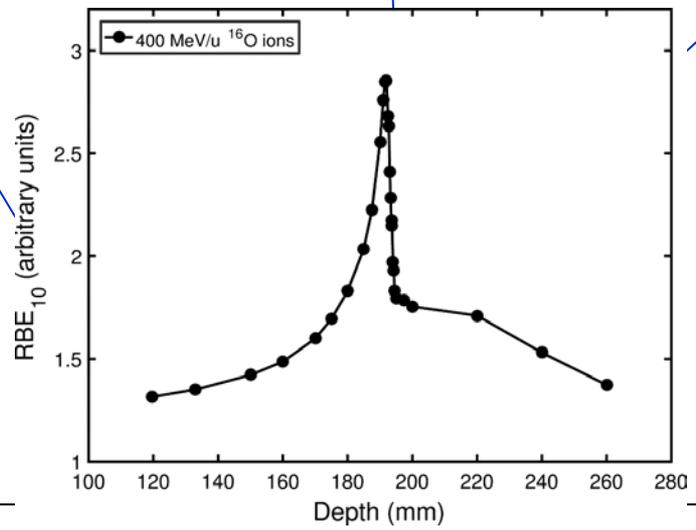
Dose mean lineal energy and  $\text{RBE}_{10}$  distribution with microdosimetric spectra for each region along the Bragg Peak
