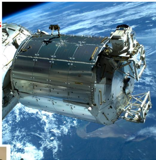
Layout of the Columbus debris shield configuration [R. Destefanis *et. al.*]
