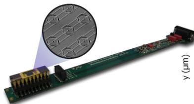
MicroPlus probe with SOI Mushroom Microdosimeter, and SEM image showing 3D sensitive volumes
