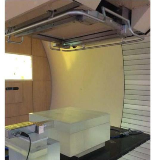
MicroPlus operates in clinical PBS with a dose rate 50-100 times higher than during the passive beam treatment delivery
