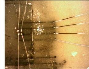
1<sup>st</sup> iteration of a diamond pixelated detector with mirrored contacts with semi-isolated sensitive volumes (2015). This concept will be extended upon in order to improve spatial resolution of ‘DiamondPix’ for particle tracking applications.
