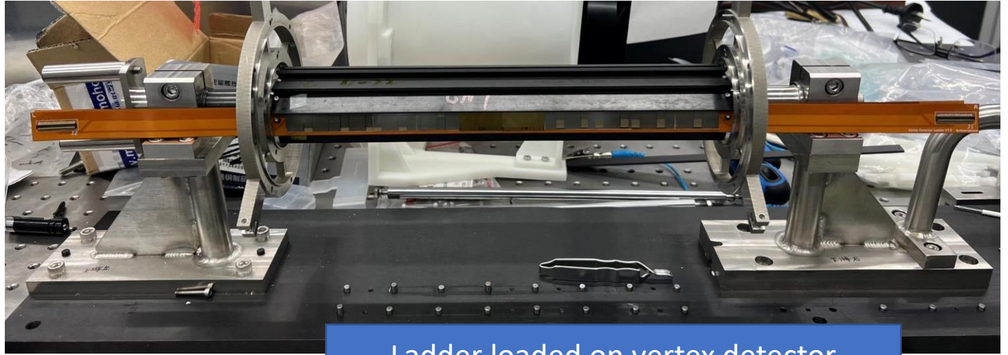
Ladder loaded on vertex detector
