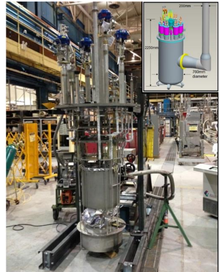
Prototype of ILC service cryostat ( 2K cooling system ; BNL )
