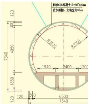
TBM tunnel (D6.5m)
