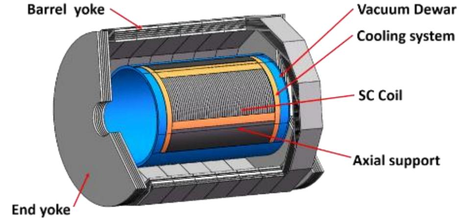
R&D: high strength HTS cable, ultra-thin cryostat.
