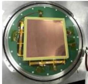
GEM-MM cathode TPC Prototype + UV laser beams
