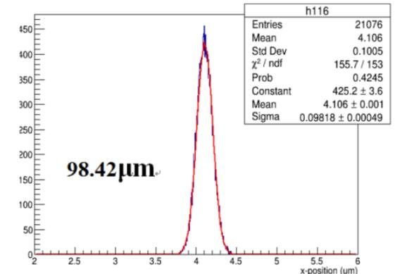
$\sigma_x < 100\ \mu\text{m}$  for drift length of 27cm
