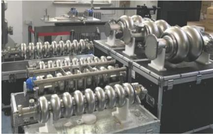
IHEP 1.3 GHz 9-cell Cavity Vertical Test
