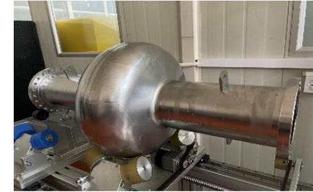
650MHz 1-cell SCRF Cavity
