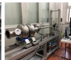
Cavity inspection camera and grinder
