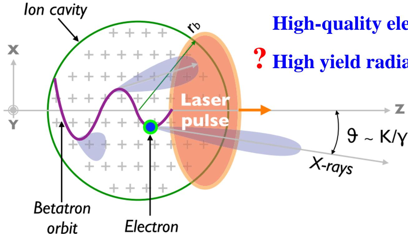
$$K = \gamma \omega_{\beta} r_{\beta} / c \simeq 1.33 \times 10^{-10} r_{\beta} [\mu\text{m}] \sqrt{\gamma n_e [\text{cm}^{-3}]}$$
