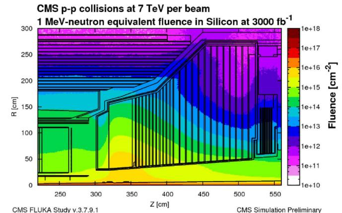
Figure 1.2: Fluence, parameterized as a fluence of 1 MeV equivalent neutrons, accumulated in HGCal after an integrated luminosity of 3000 fb<sup>-1</sup>, simulated using the FLUKA program, and shown as a two-dimensional map in the radial and longitudinal coordinates,  $r$  and  $z$ .
