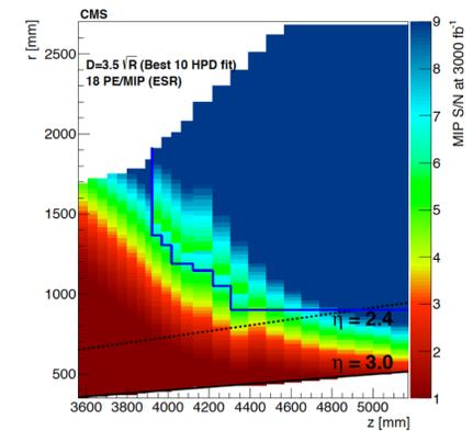
Figure 2.14: Signal-to-noise ratio for a MIP, after an integrated luminosity of  $3000 \text{ fb}^{-1}$ , shown as a two-dimensional map in  $r$  and  $z$ . The region, at larger  $z$  and  $r$ , in which SiPMs mounted on scintillator tiles can provide  $S/N(\text{MIP}) > 5$  after  $3000 \text{ fb}^{-1}$  is outlined.
