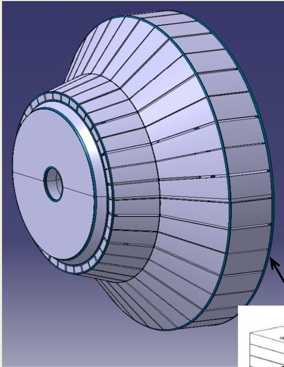
Thermal screen built from 20° wide panels, 15 – 32 mm thick depending available space
