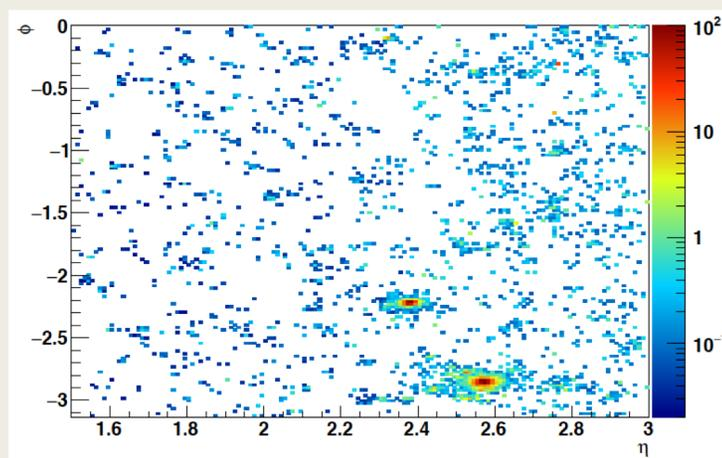
Plots show cells with  $Q > 12fC$  (threshold for timing measurement) projected to the front face of the endcap calorimeter.
