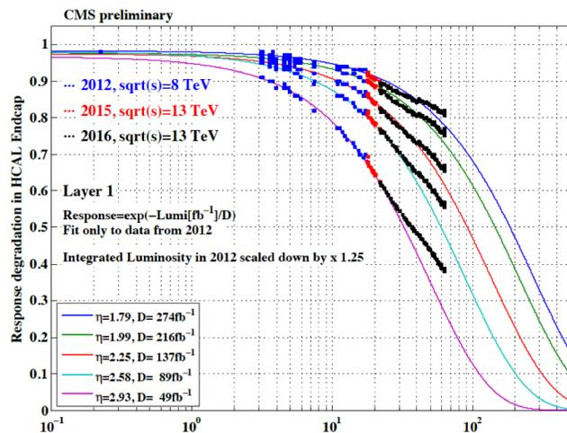
Figure 2.18: Response loss in HE Layer1 for various  $\eta$  towers, averaged over all  $\phi$  towers, as a function of integrated luminosity. The response was normalized to the signal at the beginning of 2012. The normalization for Laser intensity variation was obtained using the lowest  $\eta$  ring.
