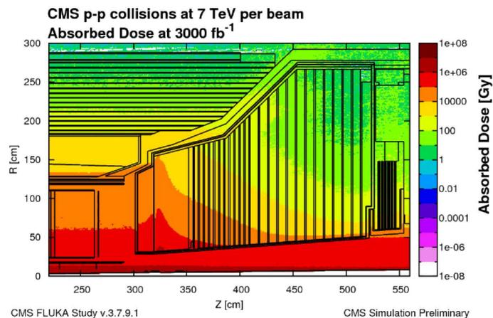
Figure 1.1: Dose of ionizing radiation accumulated in HGCal after an integrated luminosity of 3000 fb<sup>-1</sup>, simulated using the FLUKA program, and shown as a two-dimensional map in the radial and longitudinal coordinates,  $r$  and  $z$ .
