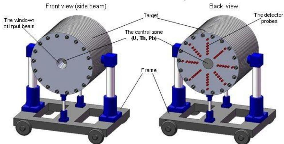
General view of the target setup BURAN at the transport-fixing platform.
