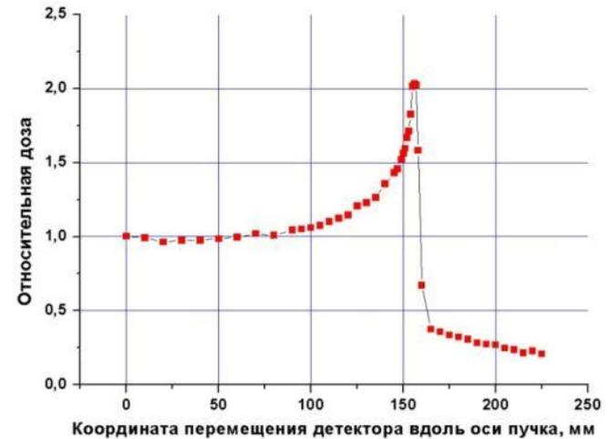
Bragg peak while moving along the beam axis diamond detector in water phantom.
