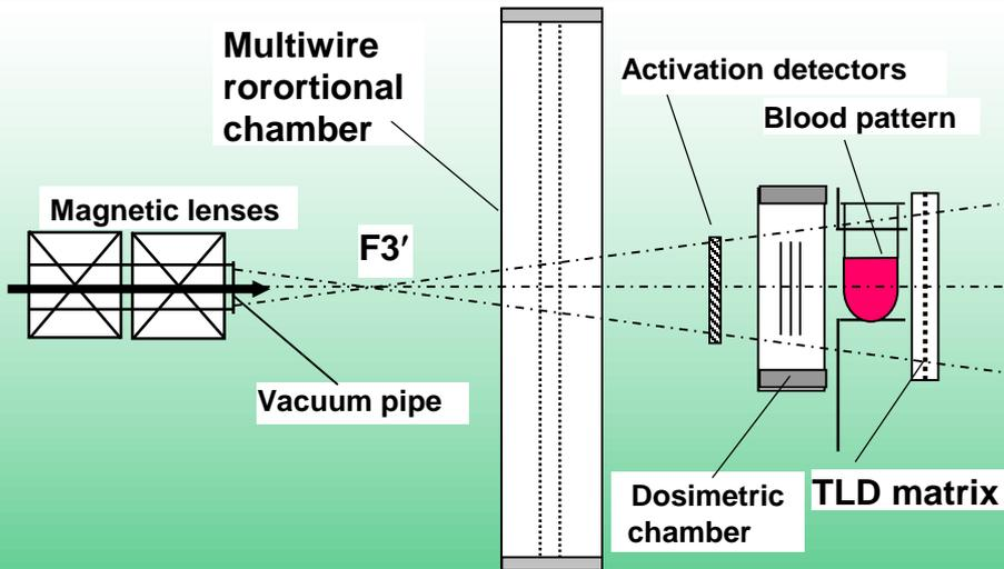
The experimental arrangement at radiobiological exposures at the Nuclotron
