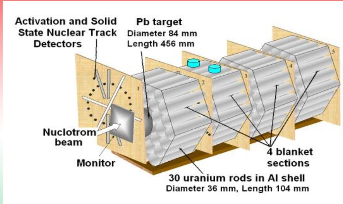
Getting new basic nuclear-physics data with relativistic proton, neutron and light ion beams **(1 - 4.5 GeV/n)** for modeling and design of the active core of the prototype for close-to-industrial setup of the radioactive waste processing
