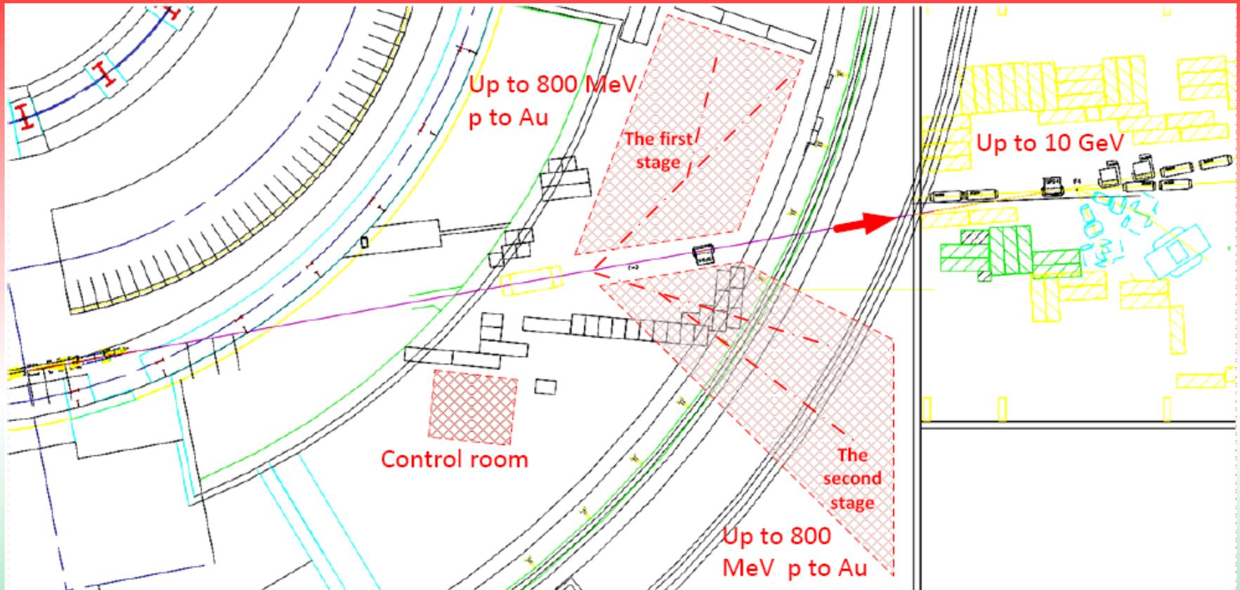
The first – the experimental setup at the gallery for the irradiation of electronics for space equipment's, materials and biological objects
