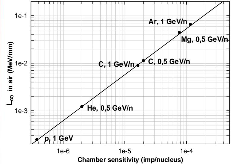
The dosimetric ionization chamber calibration at the Nuclotron beams by the activation detectors
