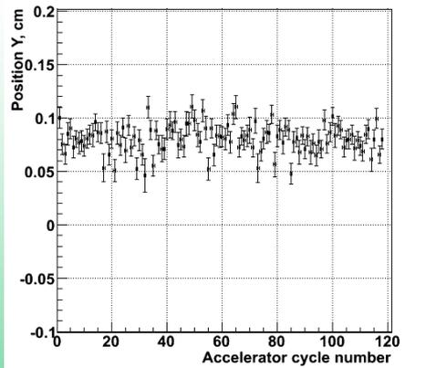
Beam position during the one irradiation run.
