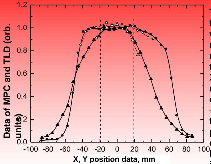
The spatial distributions of X and Y wires currents measured by the multiwire proportional chamber (● – X; ▲ – Y) and TLD readings (○ – X; △ – Y) in the formed field of 1 GeV protons. The dashed lines are the borders of the irradiation area
