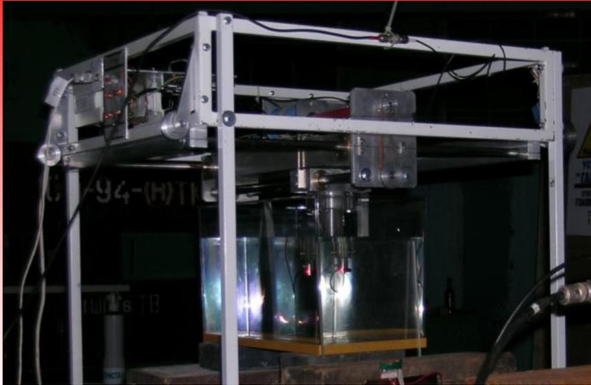
Diamond detector can be moved along and across the beam move the device with 1 mm increments. The photo shows a detector moving in the aquarium with water.
