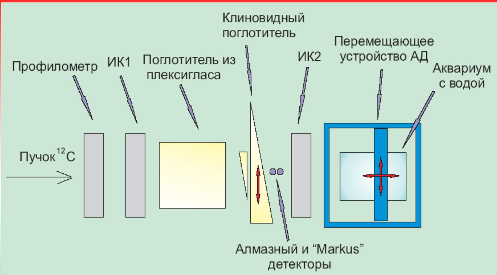
**The experimental setup "Med-Nuclotron"**
