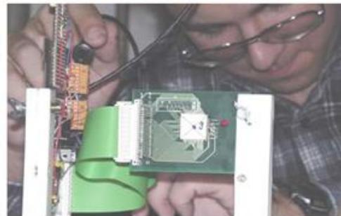
3. Radiation hardness tests
