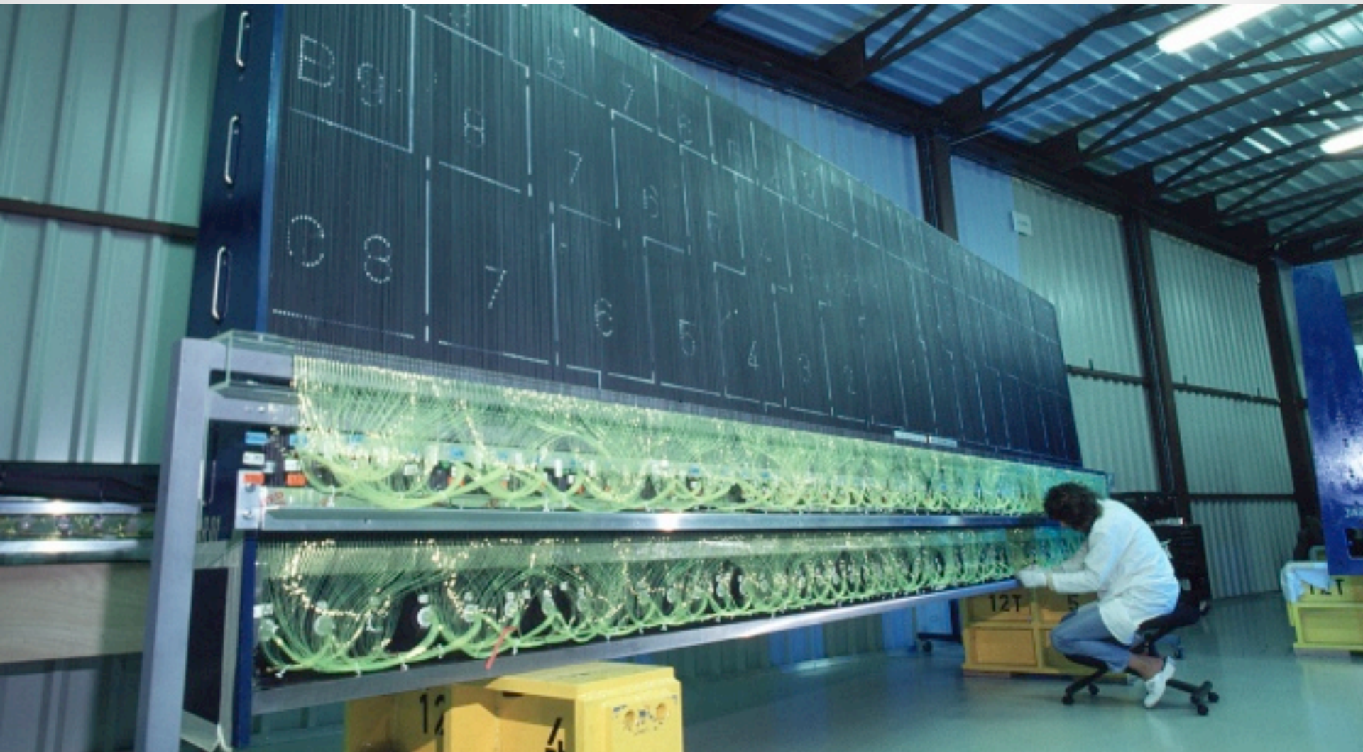
Instrumentation of the Tile Calorimeter barrel modules
