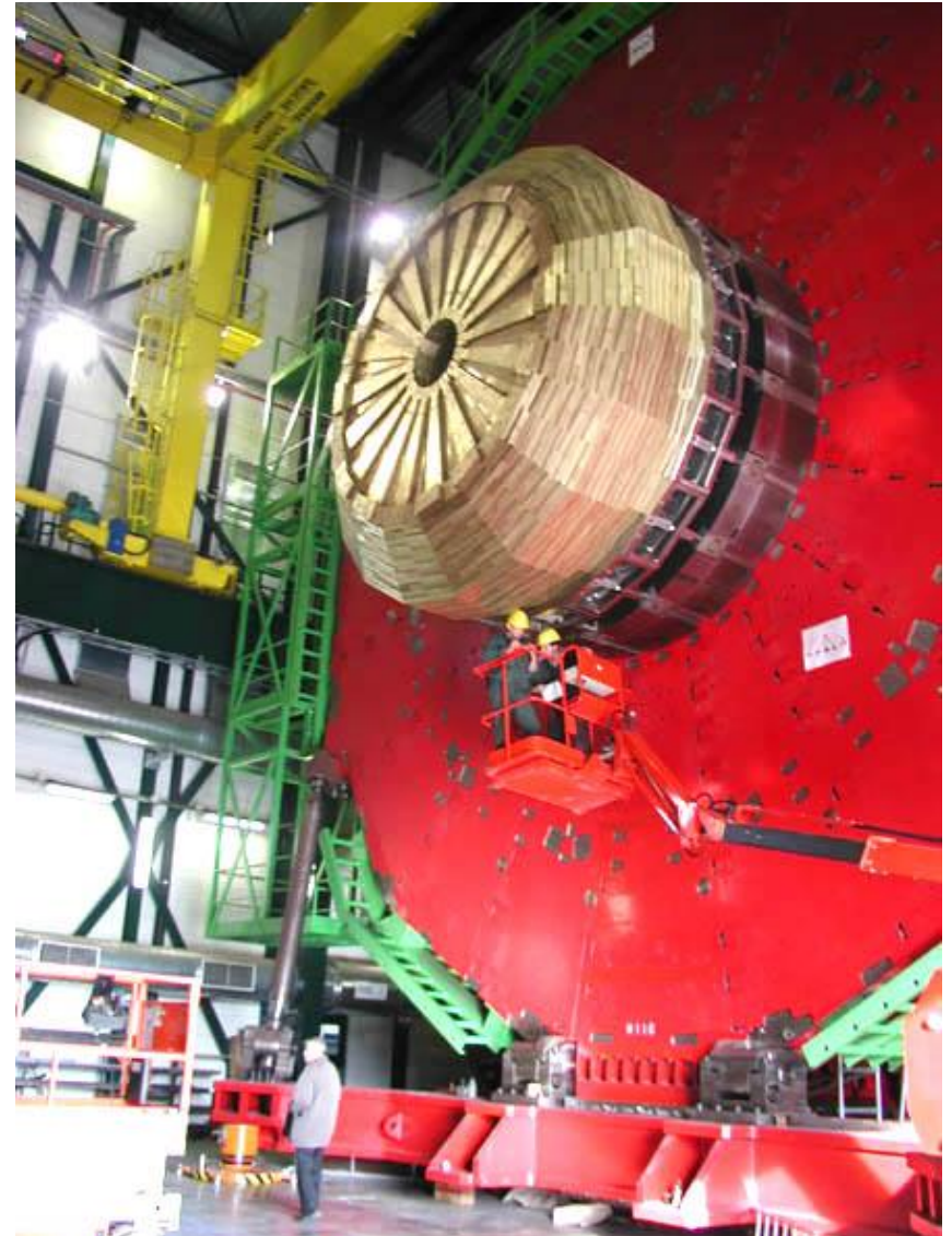
2002, CERN. Installation of CMS end-cap hadron calorimeter absorber
