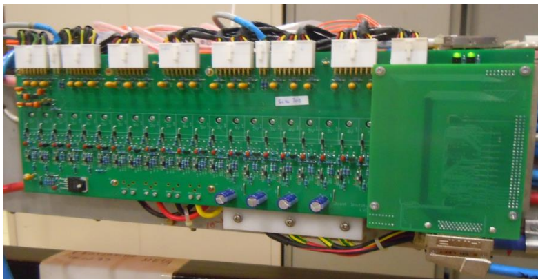
Electronic module for low voltage power supply system of CMS muon detector
