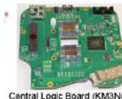
Central Logic Board (KM3NeT)
