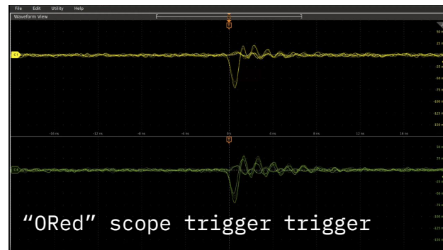
LGAD PULSE AMPLITUDE profile
