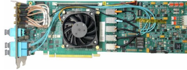
Figure 5.1: Fully assembled FLX-182 prototype card.
