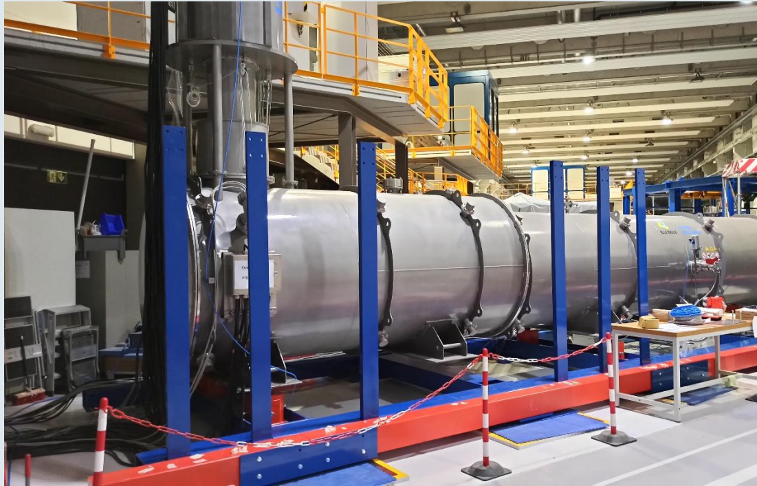
Installation of yoke frame nearing completion. Power distribution installed.
