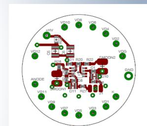
Voltage divider + preamp on Pyralux support
