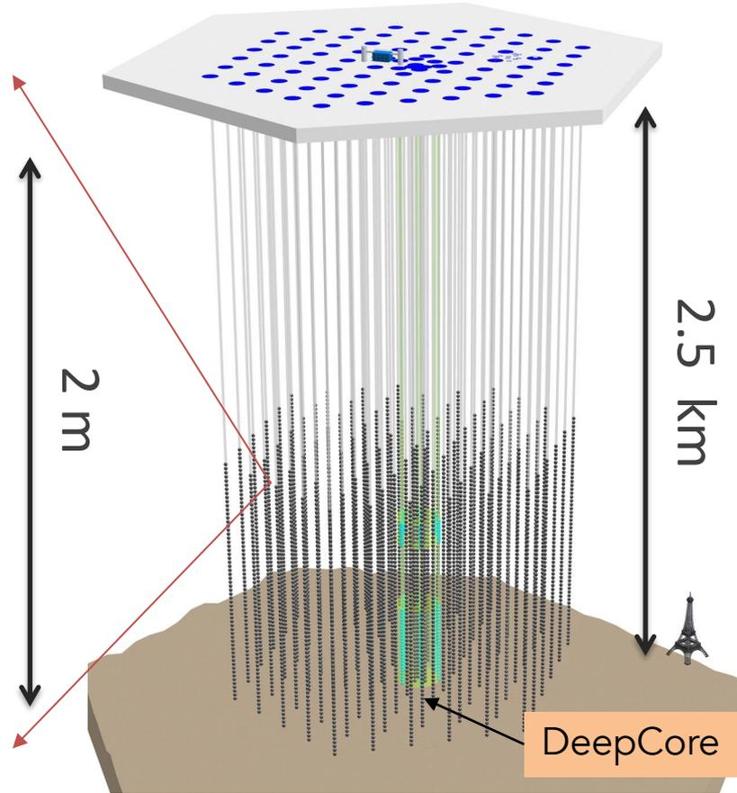
5160 DOMs spread over  $1 \text{ km}^3 = 1 \text{ Gigaton}$  instrumented volume
