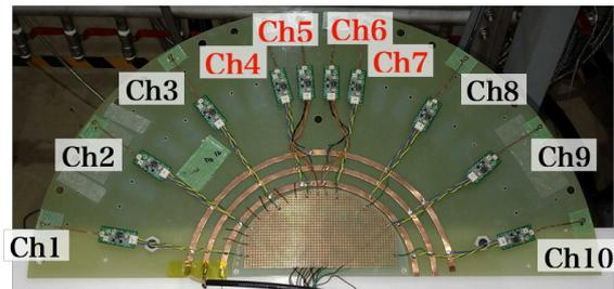
Figure 2: Prototype of multi-channel magnetic probes.
